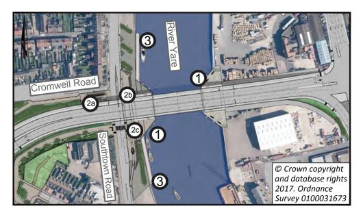
Depending on the type of bascule bridge, the bridge may need structures extending into the river to accommodate the opening mechanism (1). A control tower structure located next to the bridge would enable the 24/7 operation of the opening span. Three provisional locations have been identified for the control tower depending on the type of bascule bridge
