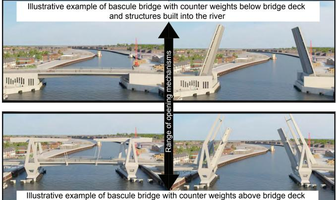
ustrative example of bascule bridge with counter weights above bridge decl and piers in the river
